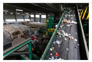
Sorting flexible plastic packaging (FPP) at the TotalRecycle material recovery facility (MRF) in Birdsboro, Penn. The Materials Recovery for the Future (MRFF) research pilot, the first of its kind in the U.S., demonstrated that FPP can be recycled through curbside recycling programs. Photo Credit: Big Foot Media, Courtesy of Nestle Purina
